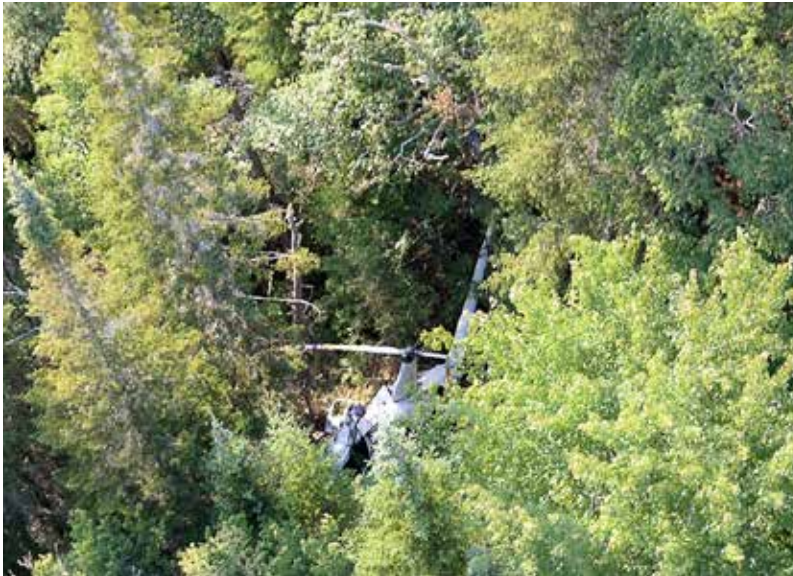
Damage to trees at the crash site indicated the accident aircraft experienced a near-vertical descent.
