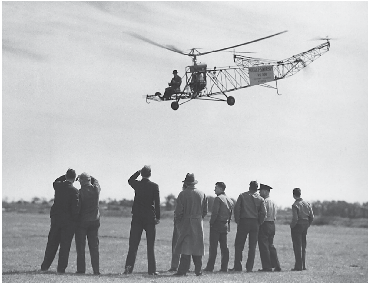
The VS-300 was modified almost daily during the early test flights that preceded its first free flight on May 13, 1940. An early major change was the addition of outrigger booms off the tail to support two small, horizontal rotors added to correct pitch and roll problems.
