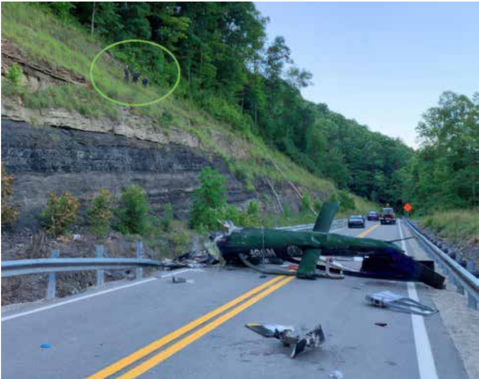
The circle at left indicates the area where the NTSB found pieces of plexiglass, the aft cap of the left skid, a tail-rotor blade segment, and green paint transfer onto a rock. (National Transportation Safety Board Photo)
